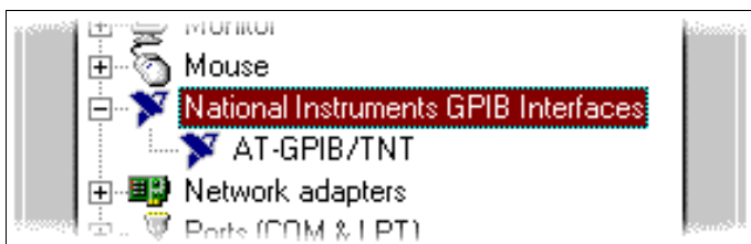
Figure 2-15. GPIB Interface That Is Working Properly
