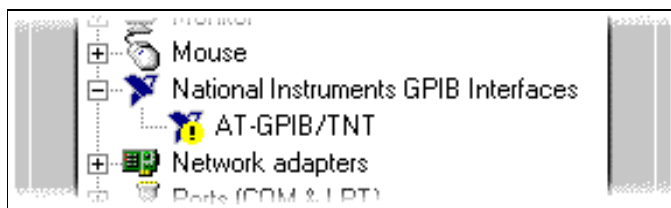
Figure C-1. GPIB Interface That Is Not Working Properly
